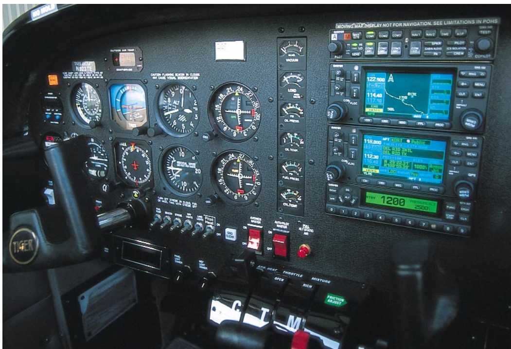
The Tiger's new all-metal instrument panel is a big step up from the original plastic ones of the '70s. This AA5B sports dueling Garmin 430s and 530s, and an energy-saving "ground" switch that fires up a single radio for clearances of GPS programming.
