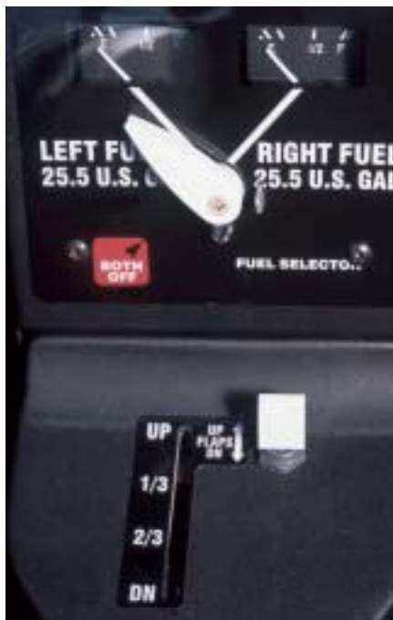
The controls for the simple fuel system sit prominently in the center console.
